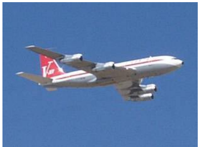
John Travolta flew a low altitude fly-by in his Boeing 707, but did not land. According to PPO Historian Mike Machat, this is a very rare model of 707, being shorter than normal and with fuel tanks for very long range, sort of like the 747SP
